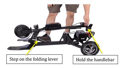
Step on the folding pedal to release the folding lock and lift the handlebar, push the handlebar forward until you hear a click, which means the folding pin is locked in securely (SNAP and GO).
