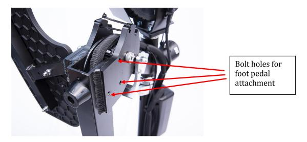
Step 2: Using the wrench, bolts and washers provided, attache the foot pedals to the flanges with the flat washer against the scooter frame and the lock washer between the flat washer and the bolt head.
