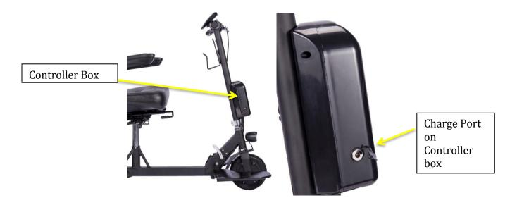
**8.** Detaching the battery: The battery comes with keys (2) to lock and unlock the battery from the scooter frame. **Please keep the spare key in a safe place. Glion does NOT have replacement keys.** Detach the charging port connecter first and then use the key provided to unlock the battery. Slide the battery out of its docking station. You can charge a detached battery using the charge port on the battery.
