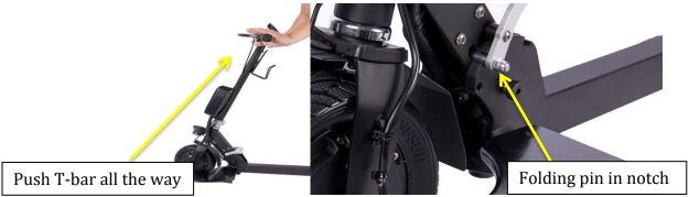
VERY IMPORTANT: Push the T-bar all the way forward and make sure the folding pin is fully seated in its notch.
