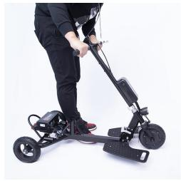
Push T-bar forward to release the pressure on locking mechanism while stepping on the folding lever. **Note:** No need to use force from foot, just rest the foot on the folding lever until the handle bar folds down.
