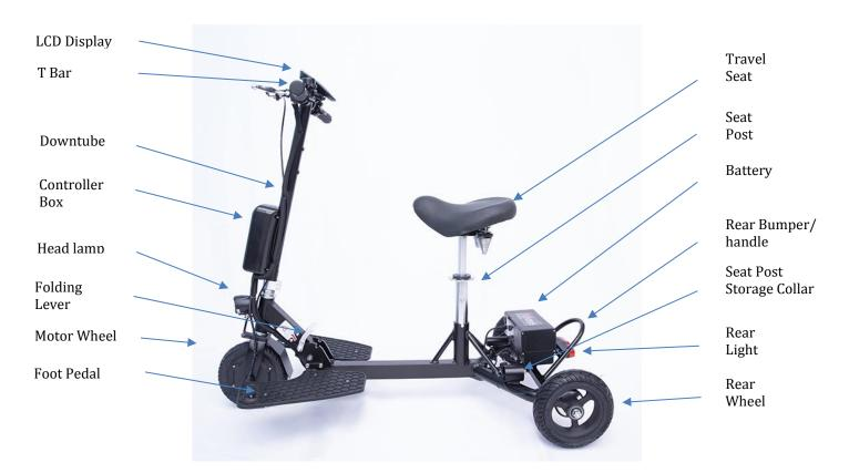
**Scooter Side View Unfolded With Travel Seat**
