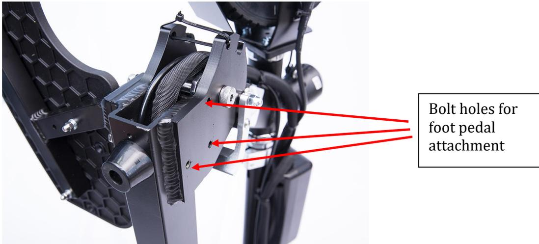
Step 2: Using the wrench, bolts and washers provided, attach the foot pedals to the flanges with the flat washer against the scooter frame and the lock washer between the flat washer and the bolt head.
