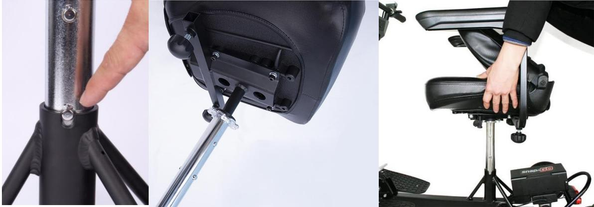
Armrest: insert the armrest in to the armrest holder under the seat. Adjust the armrest position to find the most comfortable width and use the knob to securely tighten it. You can raise and lower the armrest if needed.
