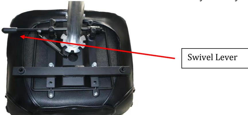
Travel Seat: Insert the seat post into the scooter frame. Then insert the travel seat into the seat post.
