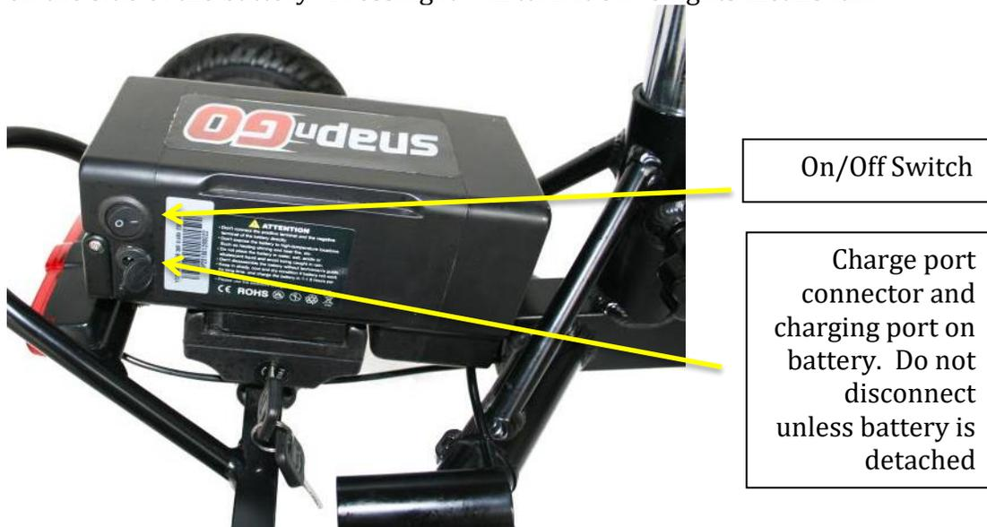
8. Detaching the battery: The battery comes with keys (2) to lock and unlock the battery from the scooter frame. **Please keep the spare key in a safe place. Glion does NOT have replacement keys.** Use the key provided to unlock the battery. Slide the battery out of its docking station. Note: To protect your investment, never detach battery and leave the exposed battery docking station in the rain. This will short and damage the battery.
