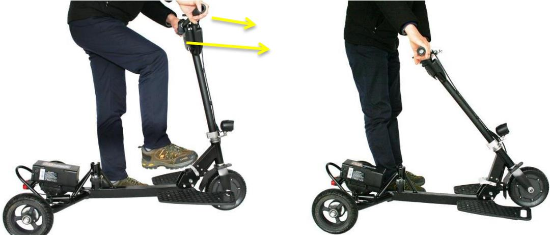
Push T-bar forward to release the pressure on locking mechanism while stepping on the folding lever. **Note:** No need to use force from foot, just rest the foot on the folding lever until the handle bar folds down.
