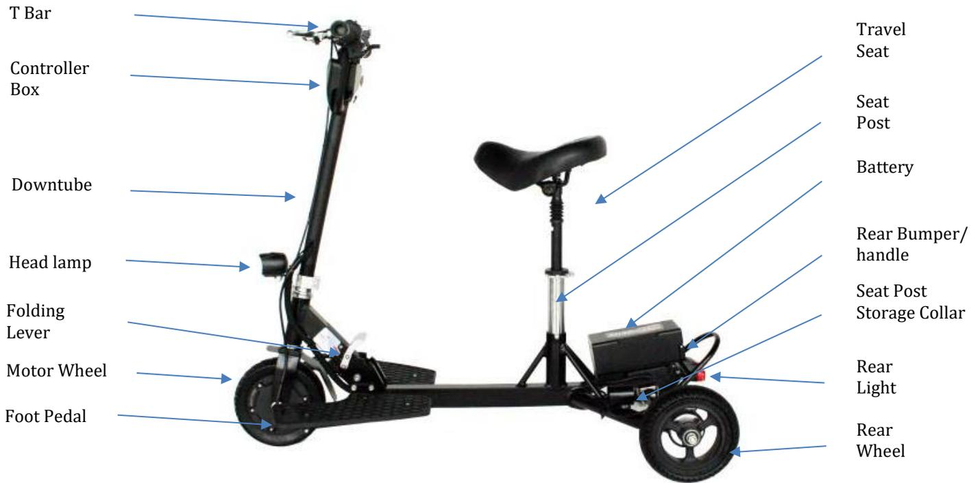
**Scooter Side View Unfolded With Travel Seat**
