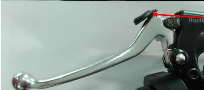
Squeeze the brake handle more and push the stopper in. Parking brake is on Gear 2. Gear 2 provides more stopping power. **For maximum stopping power, leave the scooter power on also so that front wheel electric braking is also on.**
