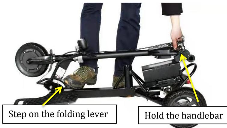
Step on the folding pedal to release the folding lock and lift the handlebar, push the handlebar forward until you hear a click, which means the folding pin is locked in securely (SNAP and GO).
