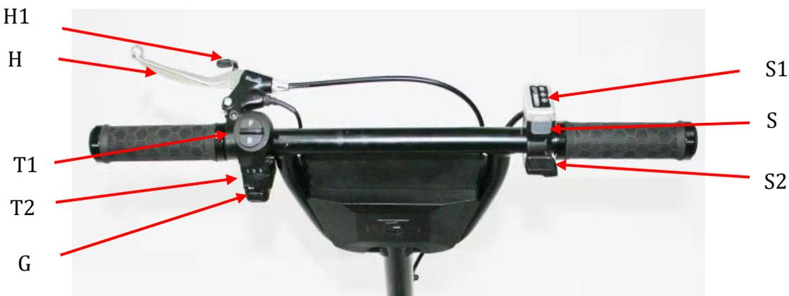
2. **Headlight On/Off:** To turn the headlight/tail on or off, you must first turn on the scooter power (S). While the scooter power is on, press the power button (S) once, the headlight and rear light should be turned on. Press (S) one more time, the headlight & rear light will be turned off.
